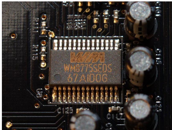
Picture 2: A Wolfson Microelectronics-made A/D converter in a circuit
